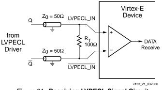
Figure 21: Receiving LVPECL Signal Circuit
