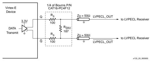
Figure 20: Transmitting LVPECL Signal Circuit
