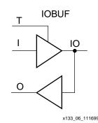
Figure 6: Input/Output Buffer Symbol (IOBUF
