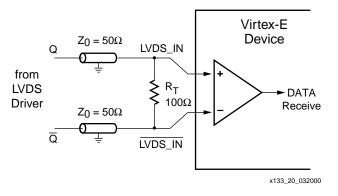
Figure 19: Receiving LVDS Signal Circuit
