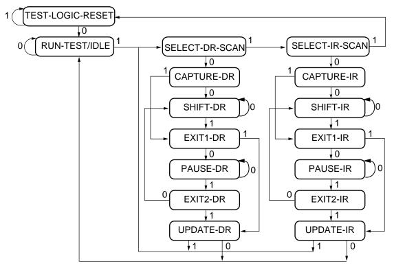
NOTE: The value shown adjacent to each state transition in this figure represents the signal present at TMS at the time of a rising edge at TCK.
