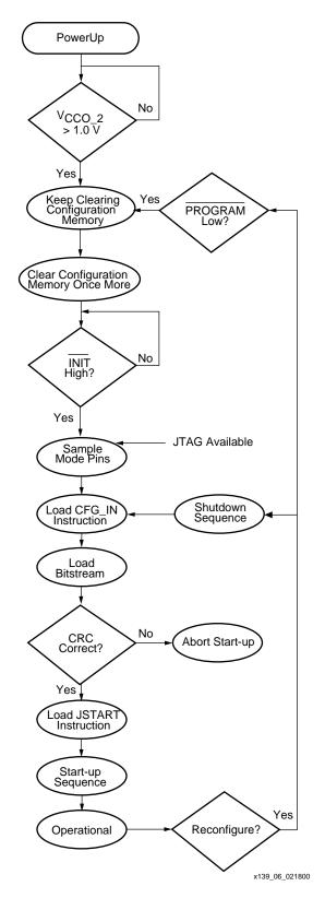
Figure 6: Device Configuration Flow Diagram
