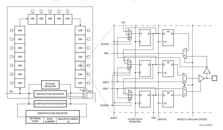
Figure 2: Virtex Series Boundary Scan Logic
