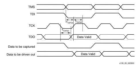
Figure 5: Virtex Boundary Scan Port Timing Waveforms
