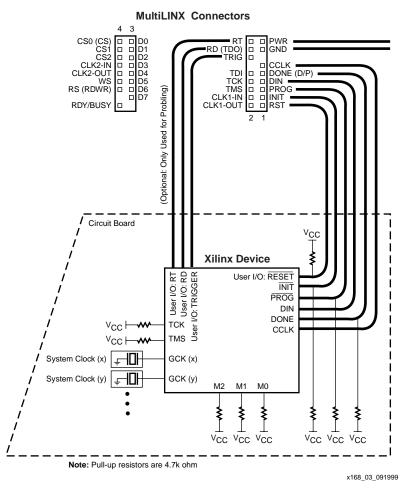
Figure 3: Serial Configuration and Verify
