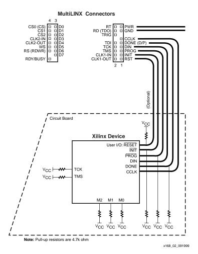
Figure 2: Serial Configuration
