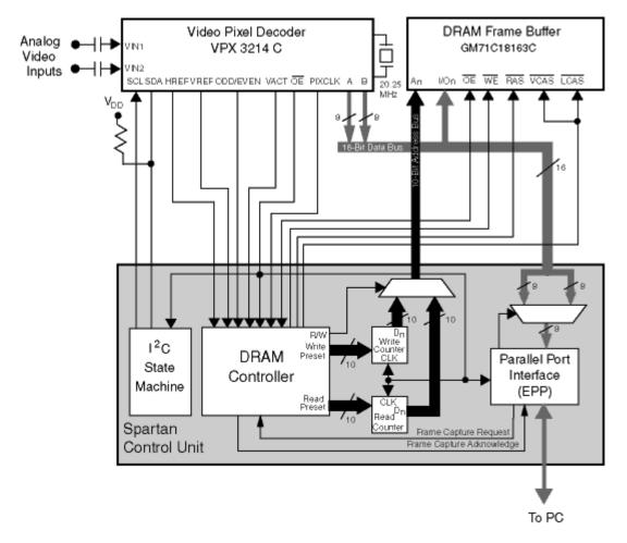
Figure 3. Detail of the Spartan Control Unit
