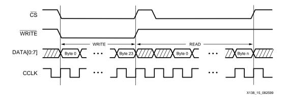
Figure 15: Readback Clocking Sequence
