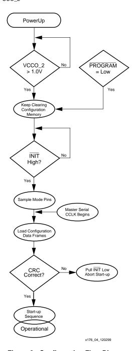
Figure 2: Configuration Flow Diagram
