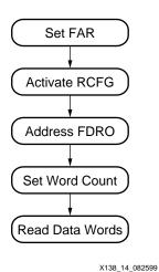
Figure 14: CLB Readback Operation Flow
