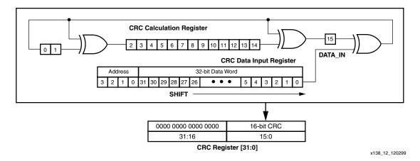
Figure 12: Serial 16-bit CRC Circuitry
