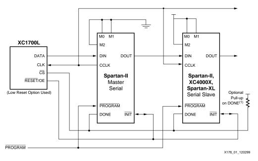
Figure 3: Master/Slave Serial Mode Circuit Diagram
