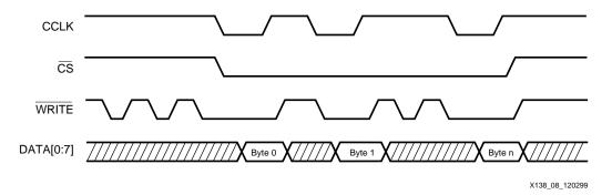
Figure 8: Controlling CCLK for WRITE De-assertion
