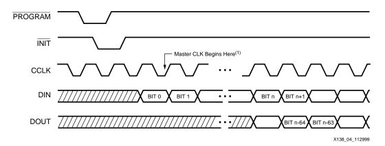
Figure 4: Serial Configuration Clocking Sequence
