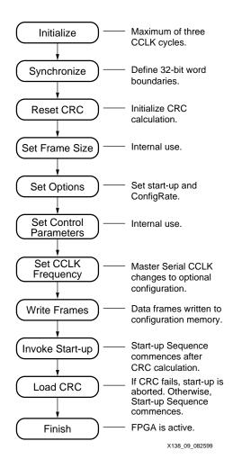
Figure 9: Internal Configuration Processing Flow
