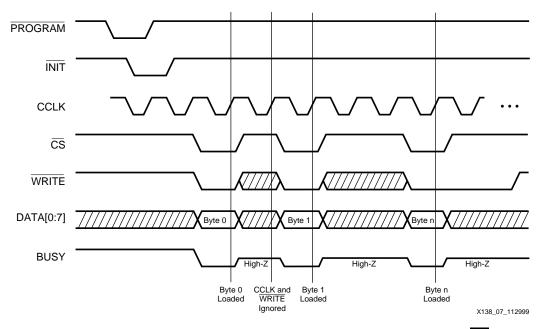
Figure 7: Separating Data Loads by Multiple CCLK Cycles Using CS
