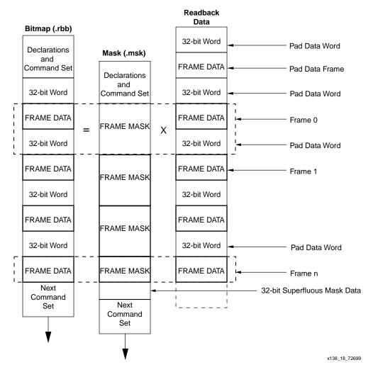
Figure 18: Readback Data Stream Alignment
