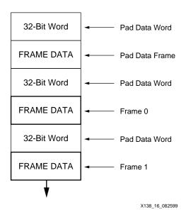
Figure 16: Readback Data Stream
