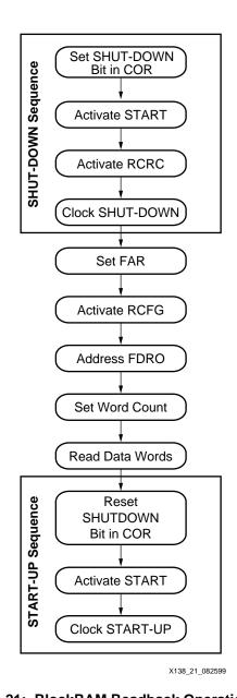
Figure 21: BlockRAM Readback Operation Flow
