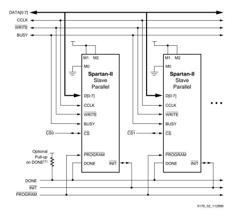
Figure 5: Slave Parallel Mode Circuit Diagram
