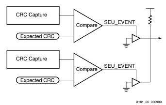
Figure 6: Redundant CRC Comparator
