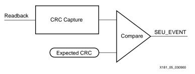
Figure 5: Readback CRCComparator
