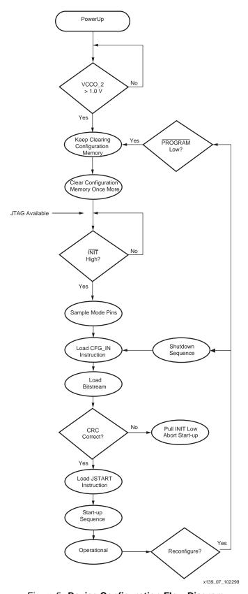
Figure 5: Device Configuration Flow Diagram
