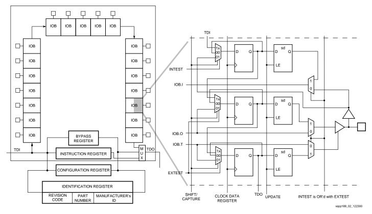
Figure 2 is a description of the Spartan-II Boundary-Scan Architecture.
