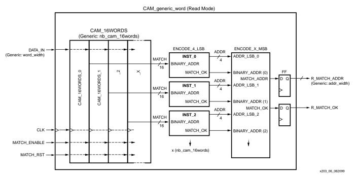
Figure 6: CAM Read Path (1 Clock Cycle)
