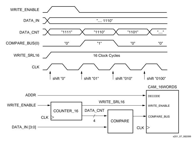
Figure 7: CAM Write Mode Waveforms
