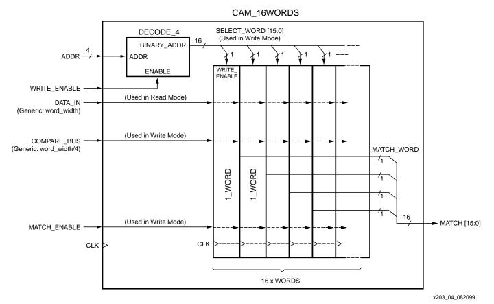
Figure 4: CAM\_16WORDS Block Diagram
