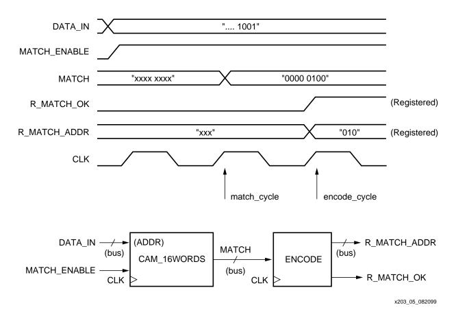
Figure 5: CAM Read Mode Waveforms
