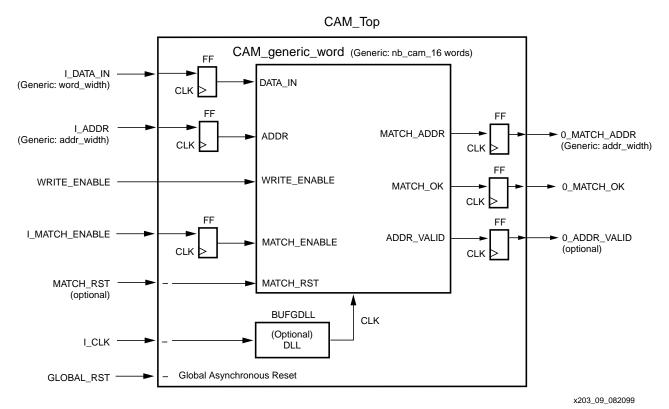
Figure 9: CAM Design Top Level Block Diagram
