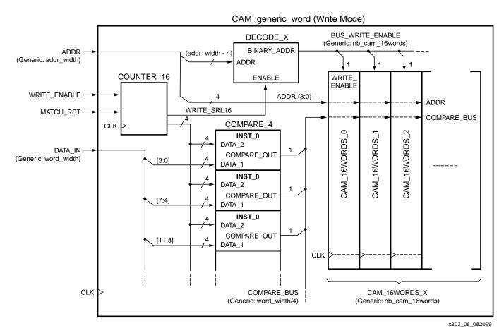
Figure 8: CAM Write Path (16 Clock Cycles to Count from 15 Down to 0)
