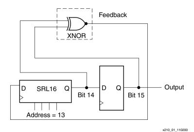
Figure 1: 15-bit LFSR Implemented Using One Slice
