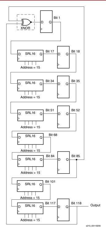
Figure 3: 118-bit LFSR Implemented Using Four Slices (2 CLBs for Virtex; 1 CLB for Virtex-II)
