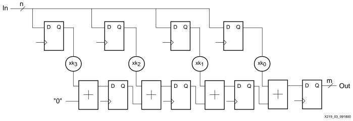
Figure 3: Transposed Form FIR Filters Employing Cascaded Pipelined Adders
