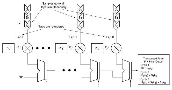
System level Z<sup>-1</sup> delay implemented by registered adders
