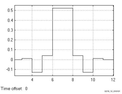
Figure 12: Ideal FIR Filter Impulse Response
