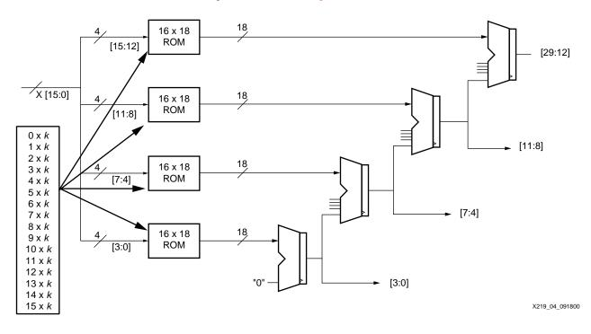
Figure 4: KCM Block Diagram
