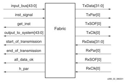
Figure 2: Top-Level CSIX Module
