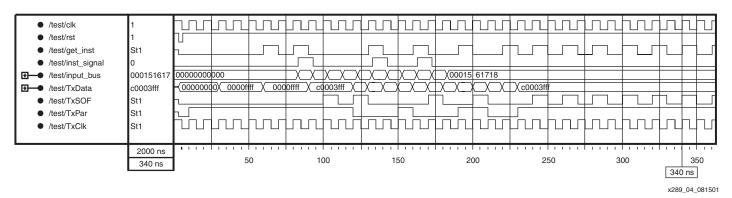
Figure 4: Transmit Signals
