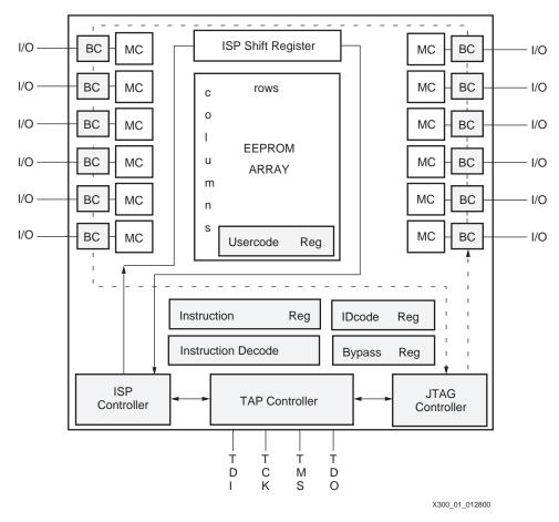
Figure 1: ISP and BST CPLD High Level Architecture
