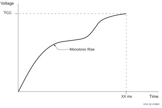
Figure 2: Realistic Voltage Ramp
