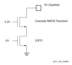
Figure 9: Cascade Connection
