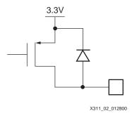
Figure 2: 5V Tolerance Incompatibility
