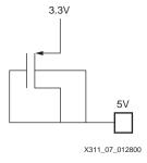
Figure 7: Equivalent PMOS Circuit
