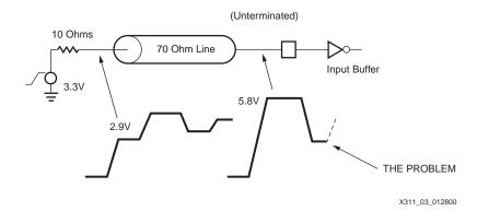
Figure 3: Unclamped Example
