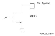
Figure 8: Typical NMOS Output Structure
