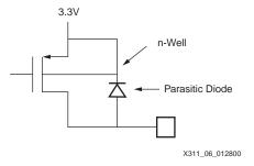
Figure 6: Output Buffer without 5V Tolerance
