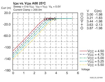
Figure 3: NMOS Output Curves
