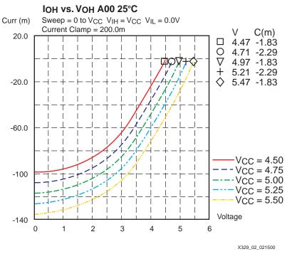
Figure 2: CMOS Output Curves
