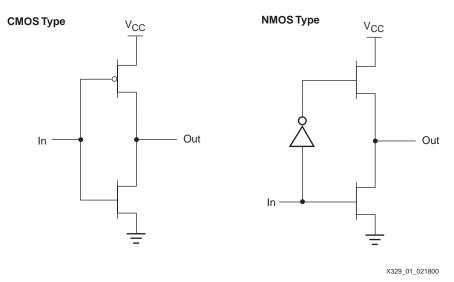
Figure 1: CMOS vs. NMOS Output Buffers
