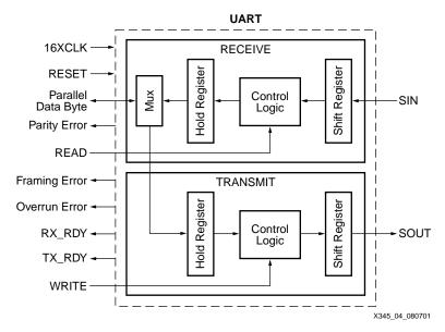
Figure 4: UART Main Interface Logic
