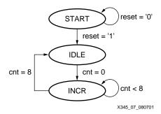
Figure 7: TXCLK Generate Logic
