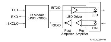
Figure 10: IR HDL Block Diagram
