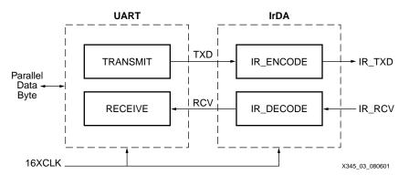
Figure 3: UART and IrDA Block Diagram
