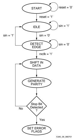
Figure 9: UART Receive Logic
