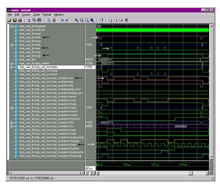
Figure 12: UART and IrDA Transmit Simulation
