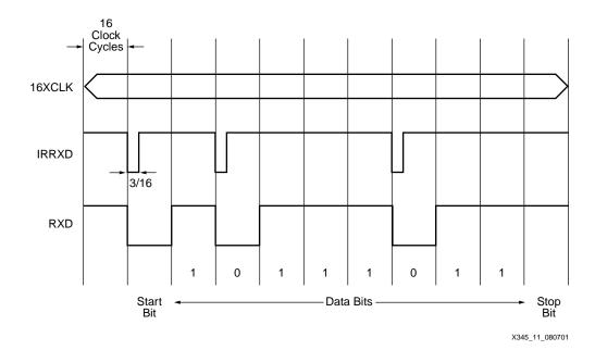
Figure 11: IrDA Decoding Scheme
