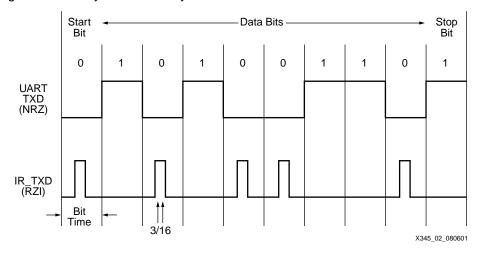
Figure 2: IrDA 3/16 Data Modulation
