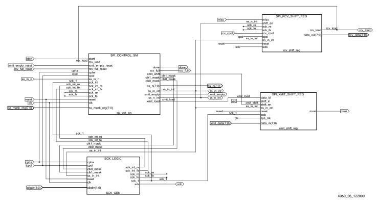
Figure 6: SPI Interface Schematic
