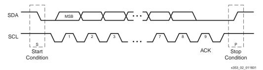
Figure 2: Data Transfer on the SMBus
