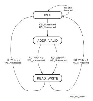
Figure 5: μC Bus Interface State Machine
