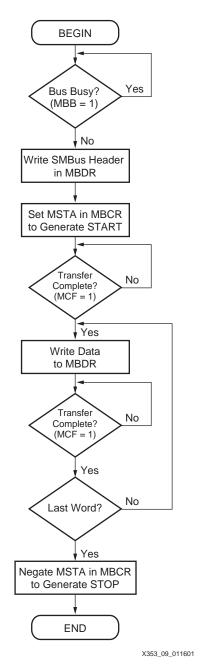
Figure 9: Master Transmit Flow Chart
