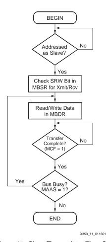
Figure 11: Slave/Transmitter Flow Chart
