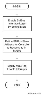
Figure 8: CoolRunner SMBus Controller Initialization Flow Chart
