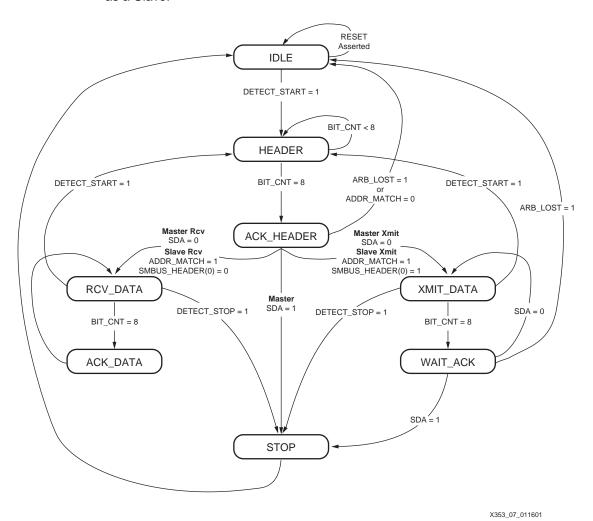
Figure 7: SMBus Interface Main State Machine
