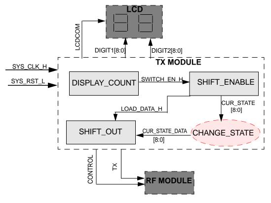
Figure 3: Transmit Module Block Diagram
