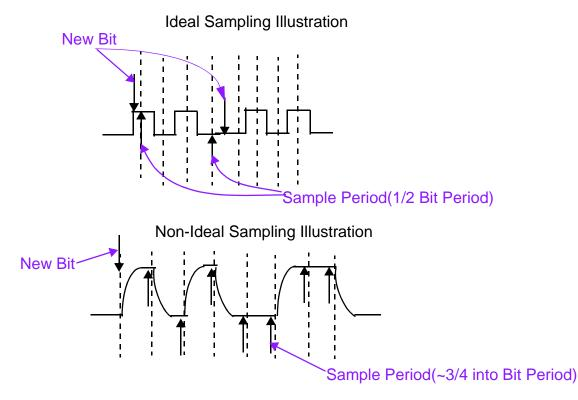
Figure 5: Receive Timing Illustrations
