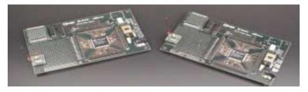
Figure 1: CoolRunner Wireless Transceiver
