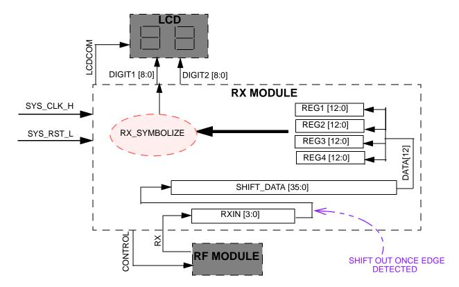
Figure 4: Receive Module Block Diagram
