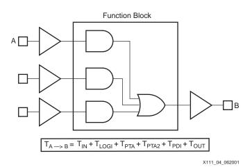
Figure 4: T<sub>PD</sub> with Initial Cascaded P-Term from Two Levels
