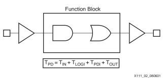
Figure 2: Simple T<sub>PD</sub> Example
