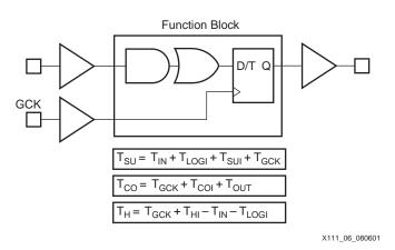
Note: Flip-flop clock-enable not shown
