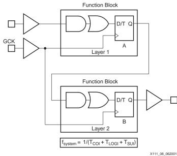
Figure 8 shows two flip-flops connected by a single level of logic, clocked by a global clock. The  $T_{SU}$  and  $T_{H}$  for flip-flop A are identical to that of Figure 6.
