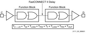
Figure 5: T<sub>PD</sub> with Multiple Pass Logic
