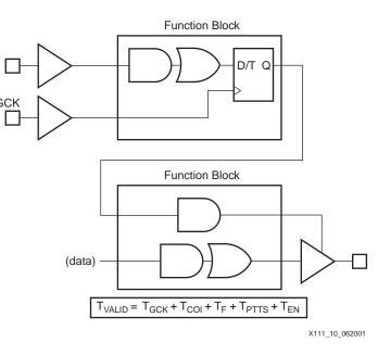
Figure 10 shows the timing for driving valid data onto a bus with respect to a rising clock edge, a common configuration that occurs in high-speed buses. This is sometimes called  $T_{VALID}$ .
