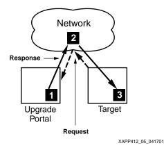
Figure 5: Pulling a payload from the upgrade portal
