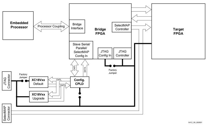
Figure 9: System with Bridge and Target FPGAs
