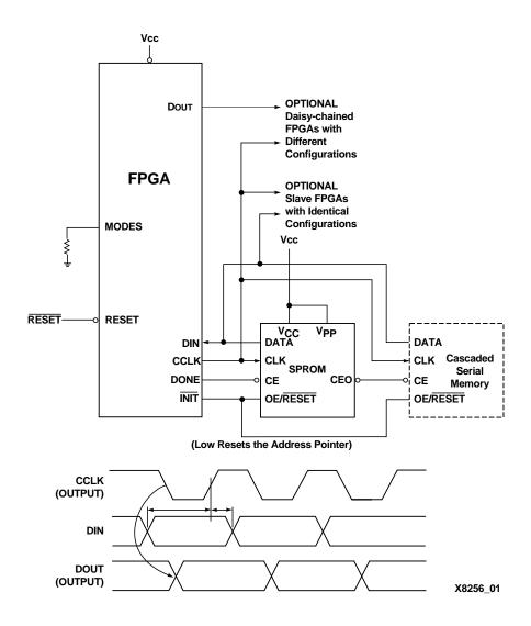
**Figure 2: Master Serial Mode.** The one-time-programmable SPROM supports automatic loading of configuration programs. Multiple devices can be cascaded to support additional FPGAs. An early DONE inhibits the SPROM data output one CCLK cycle before the FPGA I/Os become active.
