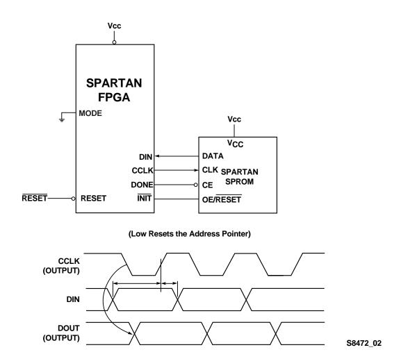
**Figure 1: Master Serial Mode.** The one-time-programmable Spartan SPROM supports automatic loading of configuration programs. An early DONE inhibits the PROM data output one CCLK cycle before the Spartan FPGA I/Os become active.
