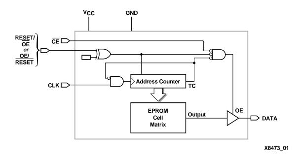
Figure 2: Simplified Block Diagram (does not show programming circuit)
