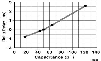
Figure 60: Delay Factor at Various Capacitive Loads
