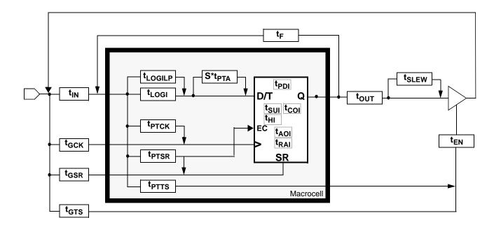
Figure 16: Detailed Timing Model
