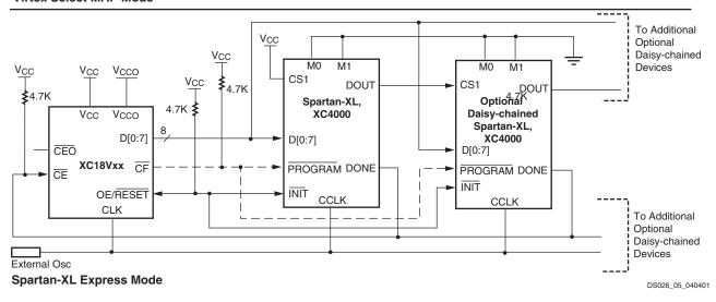
Figure 6: (a) Master Serial Mode (b) Virtex Select MAP Mode (c) Spartan-XL Express Mode (dotted lines indicate optional connection)
