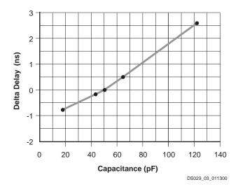
Figure 1: Delay Factor at Various Capacitive Loads
