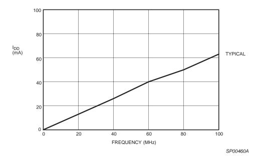
Figure 5:  $I_{CC}$  vs. Frequency @ VCC = 3.3V, 25°C
