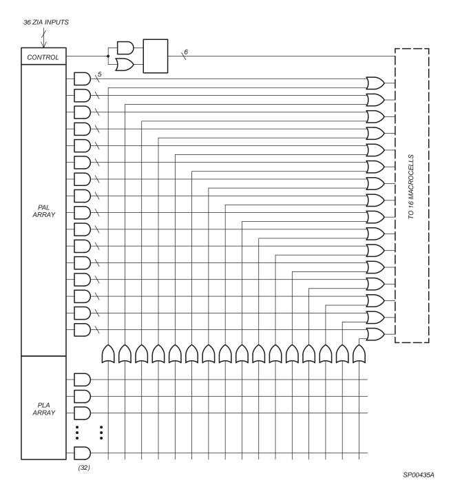
Figure 2: Xilinx XPLA Logic Block Architecture
