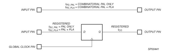
Figure 4: CoolRunner Timing Model
