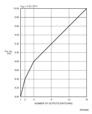
Figure 6: t<sub>PD\_PAL</sub> vs. Output Switching
