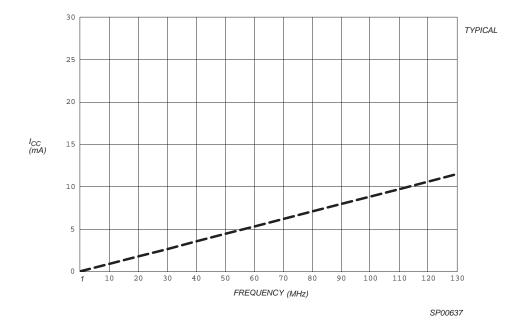
Figure 5: I<sub>CC</sub> vs. Frequency at V<sub>CC</sub> = 3.3V, 25°C
