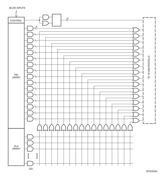
Figure 2: Xilinx XPLA Logic Block Architecture
