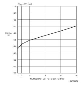
Figure 6:  $t_{PD\_PAL}$  vs. Outputs Switching
