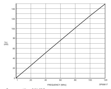
Figure 5: I<sub>CC</sub> vs. Frequency at V<sub>CC</sub> = 5.0V, 25°C
