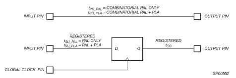
Figure 4: CoolRunner Timing Model
