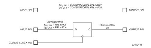
Figure 4: CoolRunner Timing Model
