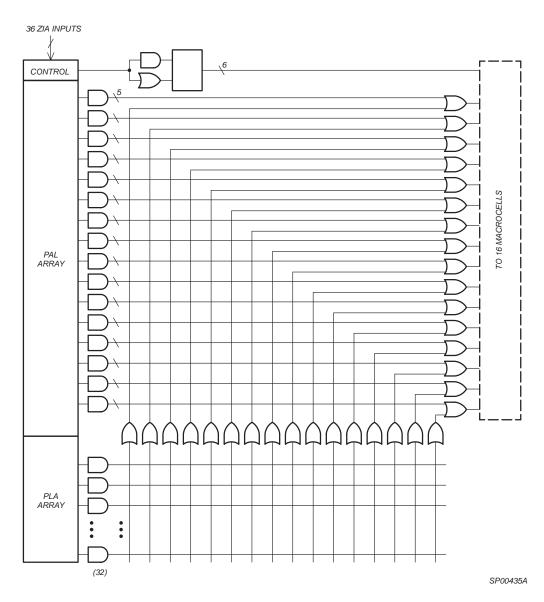
Figure 2: Xilinx XPLA Logic Block Architecture
