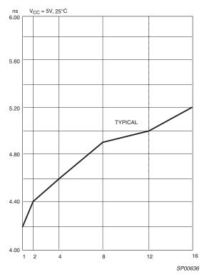
Figure 6: t<sub>PD\_PAL</sub> vs. # Outputs Switching
