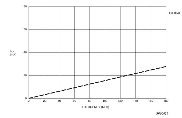
Figure 5:  $I_{CC}$  vs. Frequency at  $V_{CC}$  = 5V, 25°C
