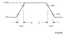
MEASUREMENTS: All circuit delays are measured at the +1.5V level of inputs and outputs, unless otherwise specified.
