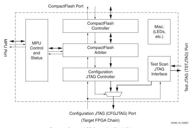
Figure 4: System ACE Controller Block Diagram
