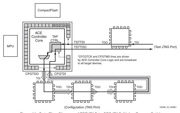
Figure 33: Data Flow Diagram of TSTJTAG to CFGJTAG (Using Bypass Path)
