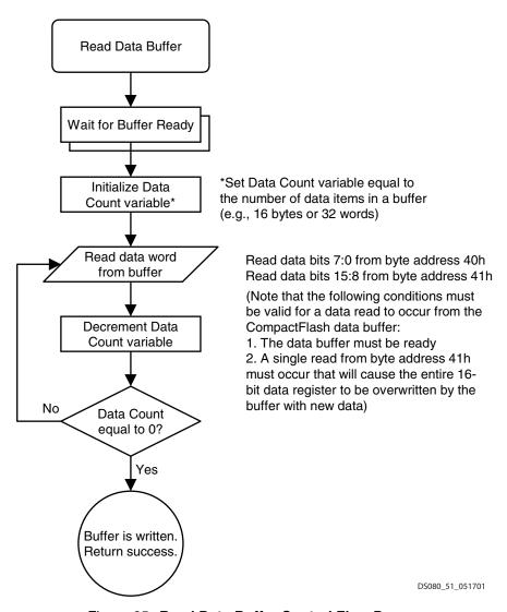
Figure 25: Read Data Buffer Control Flow Process
