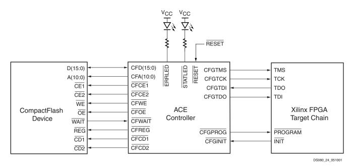
Figure 19: Wiring Diagram for CF to CFGJTAG
