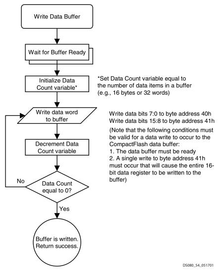
Figure 29: Write Data Buffer Control Flow Process
