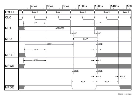
Figure 9: Single Read From an ACE Register
