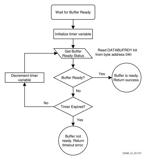
Figure 26: Wait for Buffer Ready Control Flow Process
