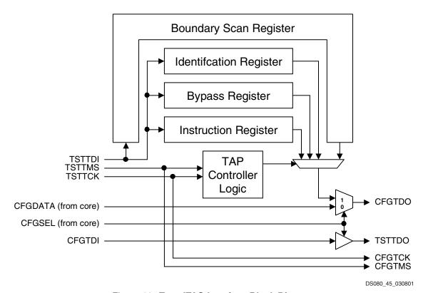
Figure 16: Test JTAG Interface Block Diagram
