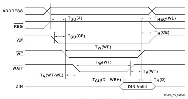
Figure 6: ACE Flash ATA Memory Write Timing Diagram
