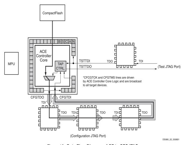
Figure 18: Data Flow Diagram of CF to CFGJTAG
