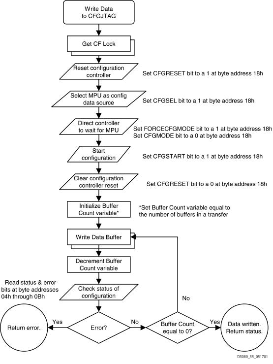
Figure 32: Write Data to CFGJTAG Interface Control Flow Process
