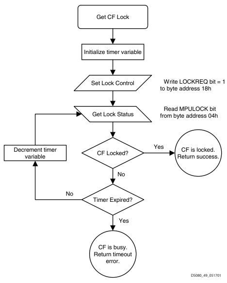
Figure 23: Get CompactFlash Lock Control Flow Process
