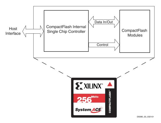
Figure 3: ACE Flash Card Block Diagram
