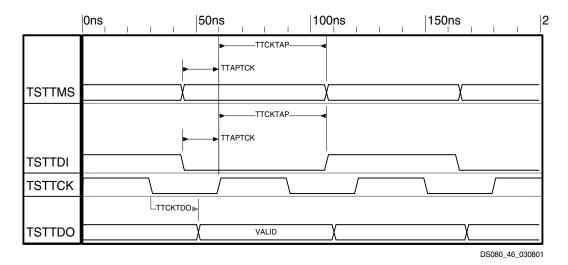
Figure 17: Test JTAG Boundary-Scan Port Timing Waveforms
