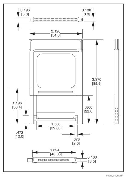
Figure 37: ACE Flash Card Adapter Dimensions
