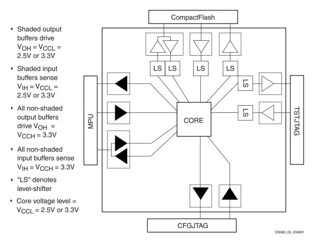
Figure 5: ACE Controller I/O Requirements
