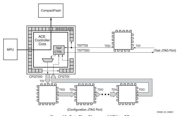
Figure 27: Data Flow Diagram of MPU to CF
