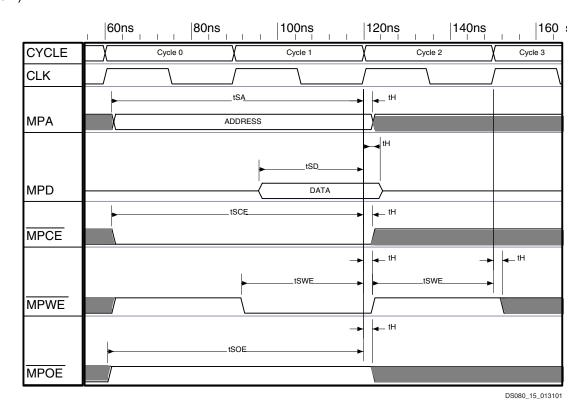
Figure 10: Single WORD Write to an ACE Register
