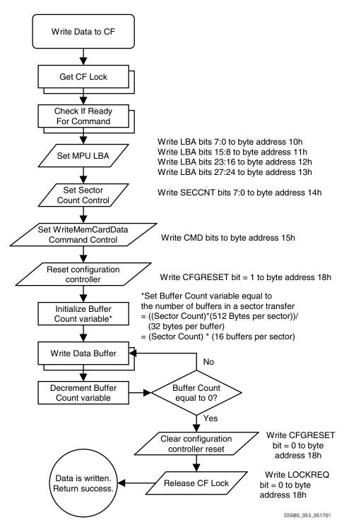
Figure 28: Write Data to CompactFlash Control Flow Process
