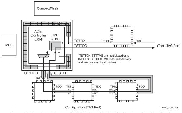
Figure 34: Data Flow Diagram of TSTJTAG to CFGJTAG (Using Boundary-Scan Path)
