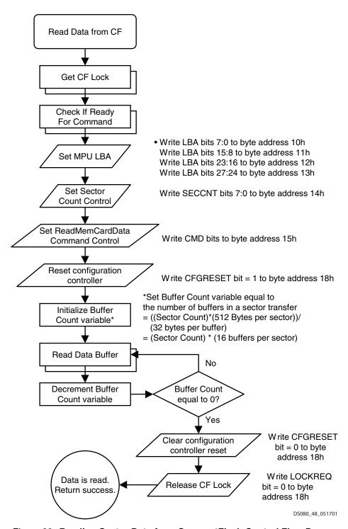
Figure 22: Reading Sector Data from CompactFlash Control Flow Process
