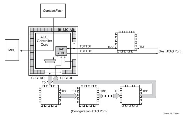
Figure 20: Data Flow Diagram of CF to MPU
