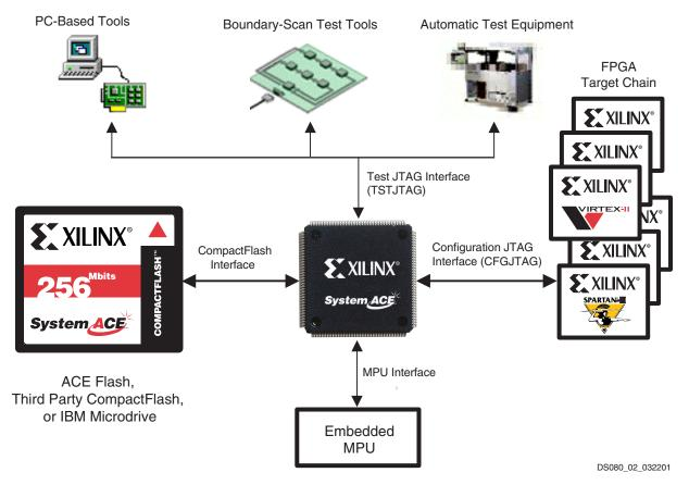
Figure 2: ACE Controller Interfaces
