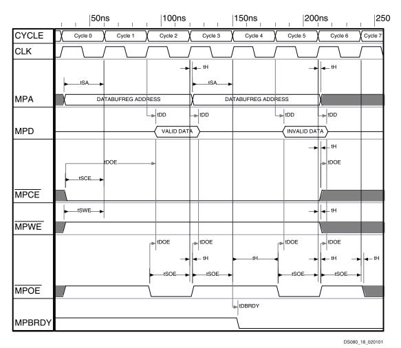
Figure 13: Valid and Invalid Reads From DATABUFREG Data Buffer
