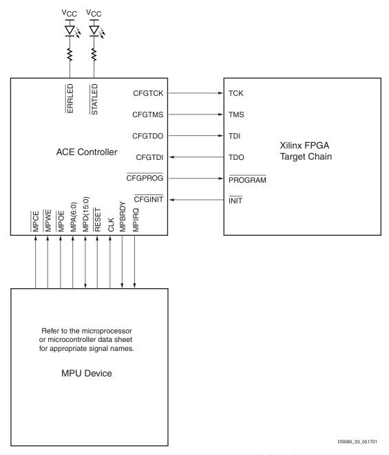
Figure 31: Wiring Diagram of MPU to CFGJTAG
