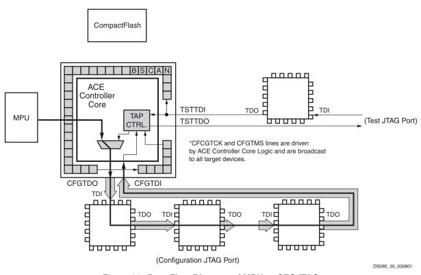
Figure 30: Data Flow Diagram of MPU to CFGJTAG
