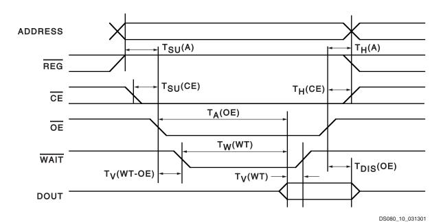
Figure 7: ACE Flash ATA Memory Read Timing Diagram
