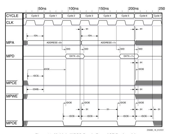
Figure 11: Multiple WORD Reads From ACE Register(s)
