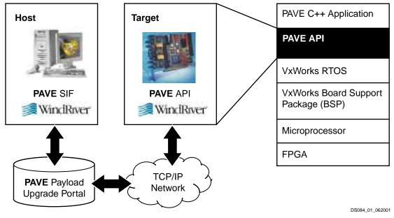
Figure 1: Xilinx PAVE in IRL Enabled System
