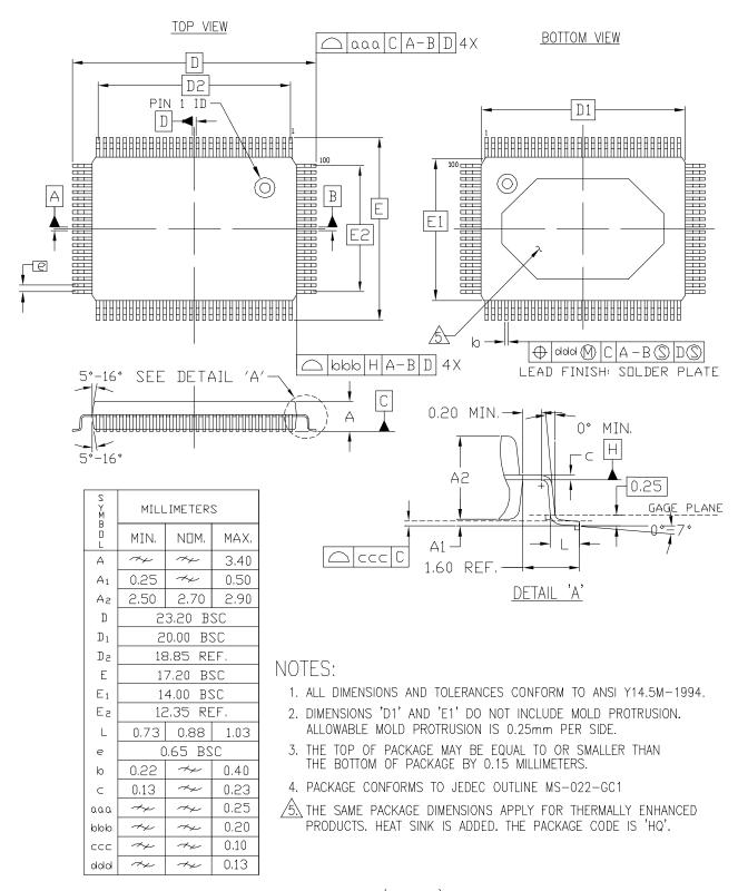
100-PIN PQFP (PQ100) 100-PIN HEAT SINK PQFP (HQ100)
