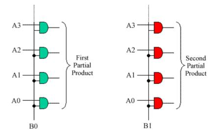
Then, we need to add all the partial products together with appropriate bit weighting. If we have time (enough clock cycles), we can adopt the classical "shift and add" technique based on an accumulator, but in this case I am looking for a maximum performance parallel multiplier. For this, I will need an "addition tree".
