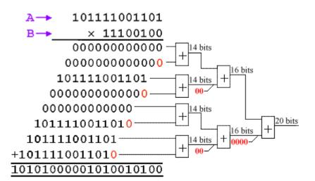
Obviously, the addition of zero bits does not require a real addition process. However, if the adder is pipelined, then the least significant bits to which zero is added will also require flip-flops to balance the pipeline delay. These flip-flops occupy the same space as a full adder (unless that wonderful SRL16E can combine several stages together).
