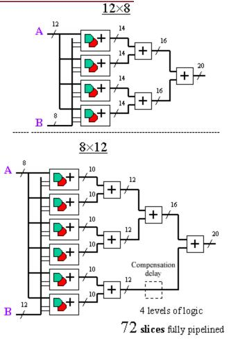
The fact that 8 is a power of 2 means that the "12x8" breaks down nicely into 4 multiplier adders in the first stage; hence, it leads to a symmetrical addition tree of 3 levels. In contrast, the "8x12" is less elegant: the 6 multiplier adders of the first stage do not sum easily, leading to more adders and 4 levels of logic. For a fully pipelined multiplier, there is even the requirement for delay compensation.
