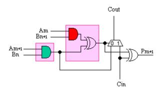
It would be nice to absorb the other AND gate into the function generator, but the signal it produces is also required by the MUXCY part of the addition function. So this would appear to be the most we can achieve.
