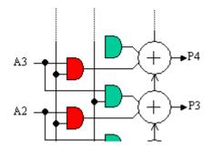
However, we can quickly see an optimisation. The AND gate associated with one of the adder inputs can be absorbed into the function generator forming the Half\_sum for addition. This in itself reduces the size of the 12-bit by 8-bit multiplier by 48 function generators (24 slices).
