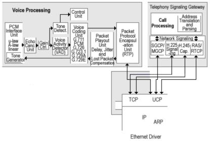
Figure 2: VoIP Gateway Architecture
