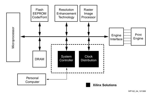
Figure 4: Printer Controller Block Diagram
