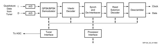
Figure 3: Decoder Block Diagram
