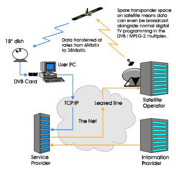
Figure 1: Internet Access Network Architecture (Courtesy of the DVB Project)
