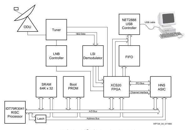
Figure 4: HNS DirecPC®-USB Receiver Block Diagram
