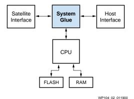
Figure 2: Satellite Modem Architecture
