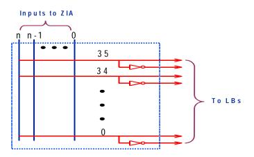
Figure 6: XPLA3 Zero Power Interconnect Array (ZIA)
