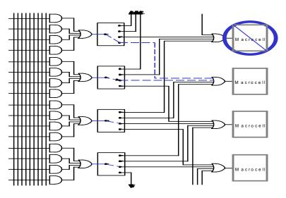
Figure 13: Logic Block Architecture with Product-term Steering
