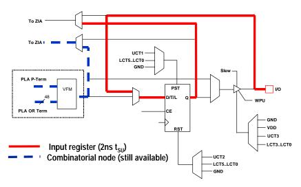
Figure 16: XPLA3 Input Register
