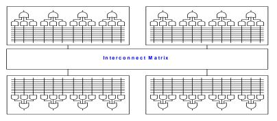
Figure 3: Basic CPLD Architecture
