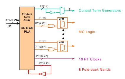
Figure 7: XPLA3 Logic Block Architecture
