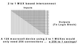
Figure 5: 2:1 Mux Based Interconnect
