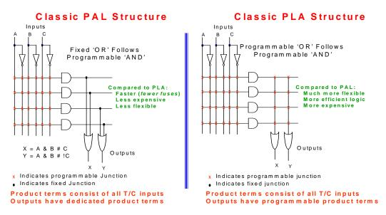
Figure 11: Basic PAL / PLA Structures
