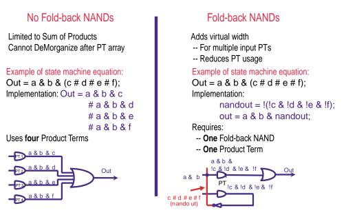
Figure 10: Fold-back NAND Design Example
