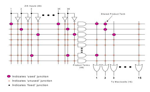
Figure 14: XPLA3 Logic Block with Pure PLA Array
