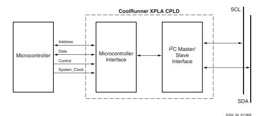
Figure 3: CoolRunner I<sup>2</sup>C Bus Controller
