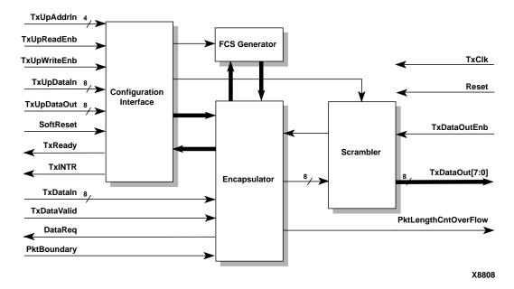
Figure 2: CC318f Transmitter Block Diagram (Courtesy: CoreEL Microsystems)
