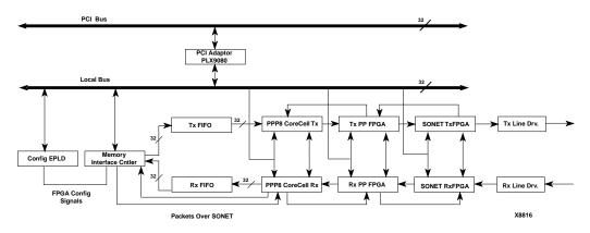
Figure 4: Application of HDLC PPP Cores (Courtesy: CoreEL MicroSystems)
