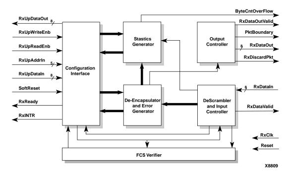
Figure 3: CC318f Receiver Block Diagram (Courtesy: CoreEL Microsystems)
