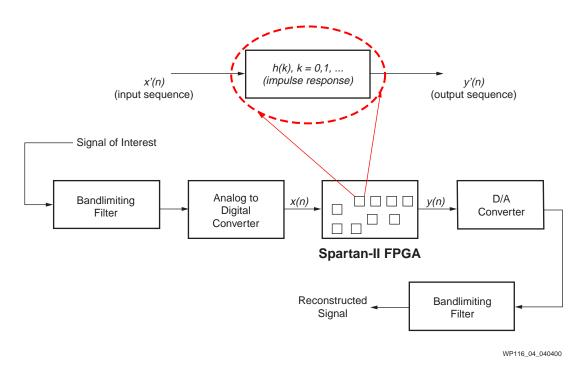
Figure 4: FIR Filter(s) in an Application
