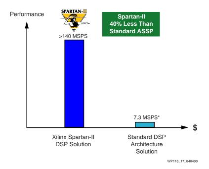
Figure 17: Spartan-II Advantage over DSP Implementation of FIR Filter
