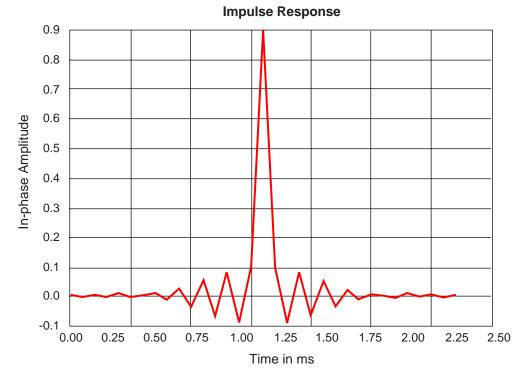
Figure 7: Impulse Response Plot of the Calculated Low-Pass Filter Using Windowing
