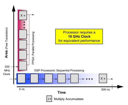
Figure 12: FPGA vs. DSP Architecture – Solution Implementation
