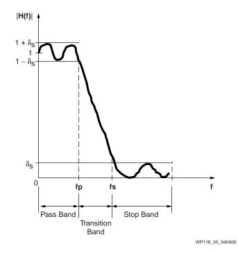
Figure 5: Example Showing Filter Requirements for a Low Pass Filter
