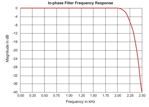
Figure 6: Magnitude Plot of the Calculated Low-Pass Filter Using Windowing
