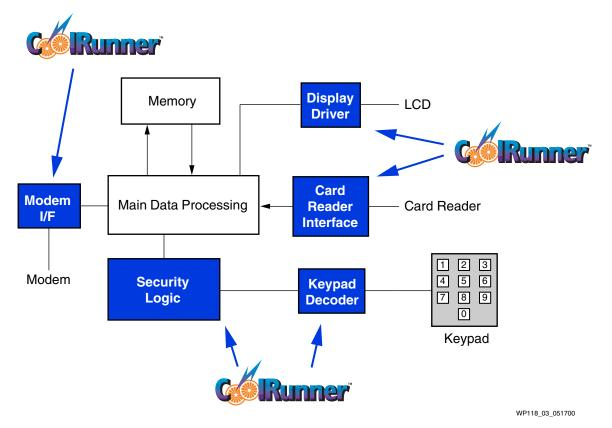
Figure 3: Example of a Smart Card Reader Internal Functions
