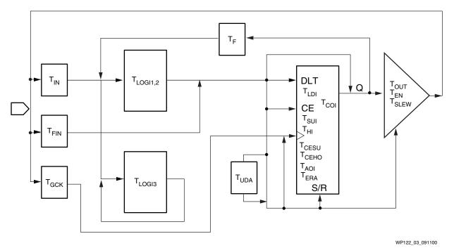
Figure 3: XPLA3 Detailed Timing Model
