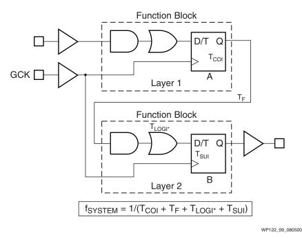
Figure 9 shows two flip-flops connected by a single level of logic, clocked by a global clock. The  $T_{SU}$  and  $T_{H}$  for flip-flop A are identical to that of Figure 7.
