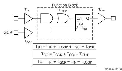
Figure 7: Simple Flip-Flop Path
