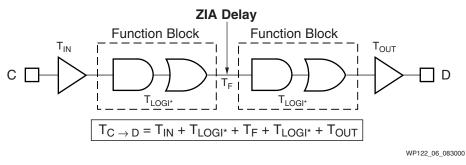
Figure 6: T<sub>PD</sub> with Two-Pass Logic
