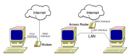
Figure 1: Application of Digital Modems and SOHO Routers
