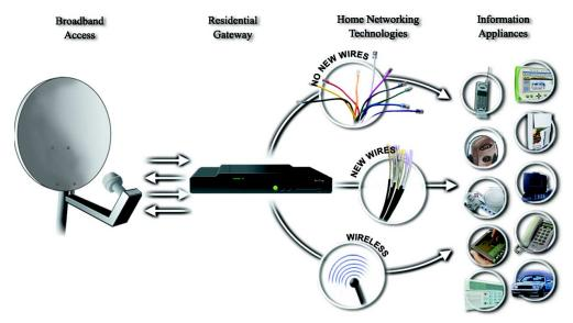
Figure 3: Architecture of a Home Network
