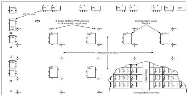
Figure 5: Generic FPGA Architecture
