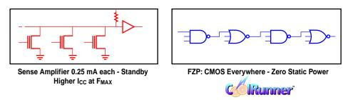
Figure 2: Sense Amplifier and Fast Zero Power for CoolRunner CPLDs
