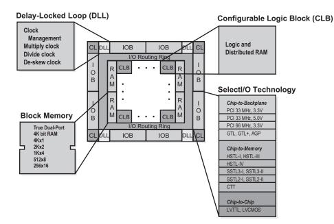
Figure 6: Architecture and Feature Overview of the Spartan-II Family
