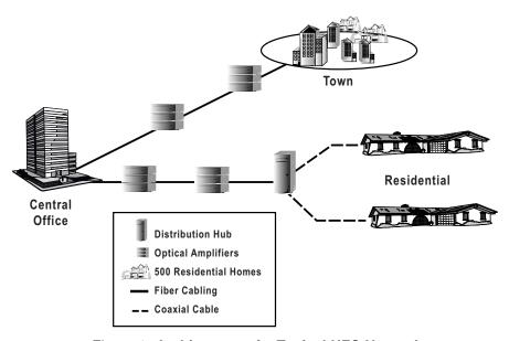
Figure 1: Architecture of a Typical HFC Network
