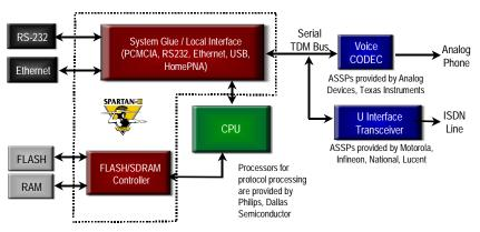
Figure 4: ISDN Modem
