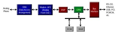
Figure 5: Analog Modem
