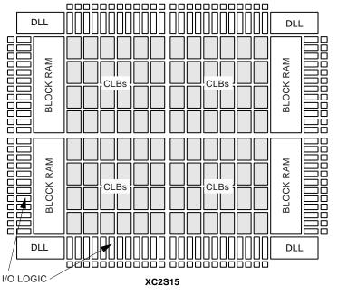
Figure 1: Architecture on Spartan-II FPGAs
